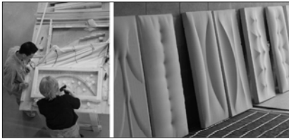
Figure 1. Model formwork and completed plaster casts (C.A.S.T. photos).
