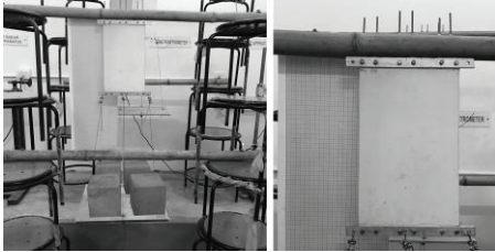
Figure 4: Test setup for measuring creep in fabric
