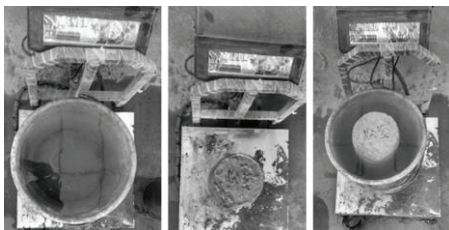
Figure 10: Setup to measure density of concrete
