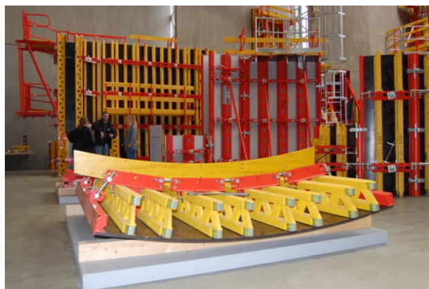
Fig. 4: Photo showing PERI's single curvature scaffolding.
