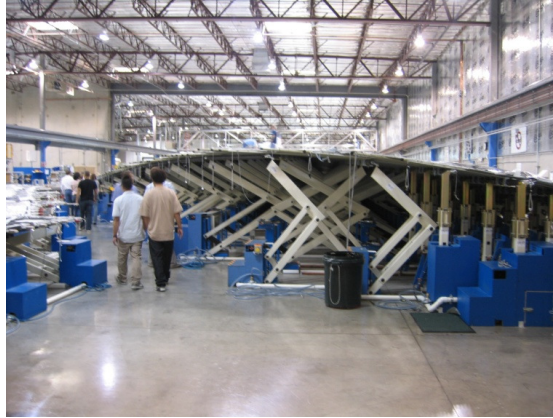
Fig. 7: North Sails mould with numerous actuators.
