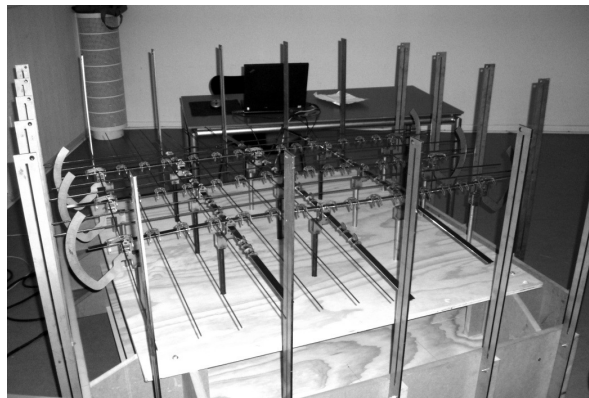
Fig. 10: The structure connecting the membrane to the actuators consists of spring steel members that are allowed to slide in both directions to obtain the movements of the flexible membrane. The system is designed to ensure, that the surface of the membrane has a constant offset from the surface defined by the actuator heads.
