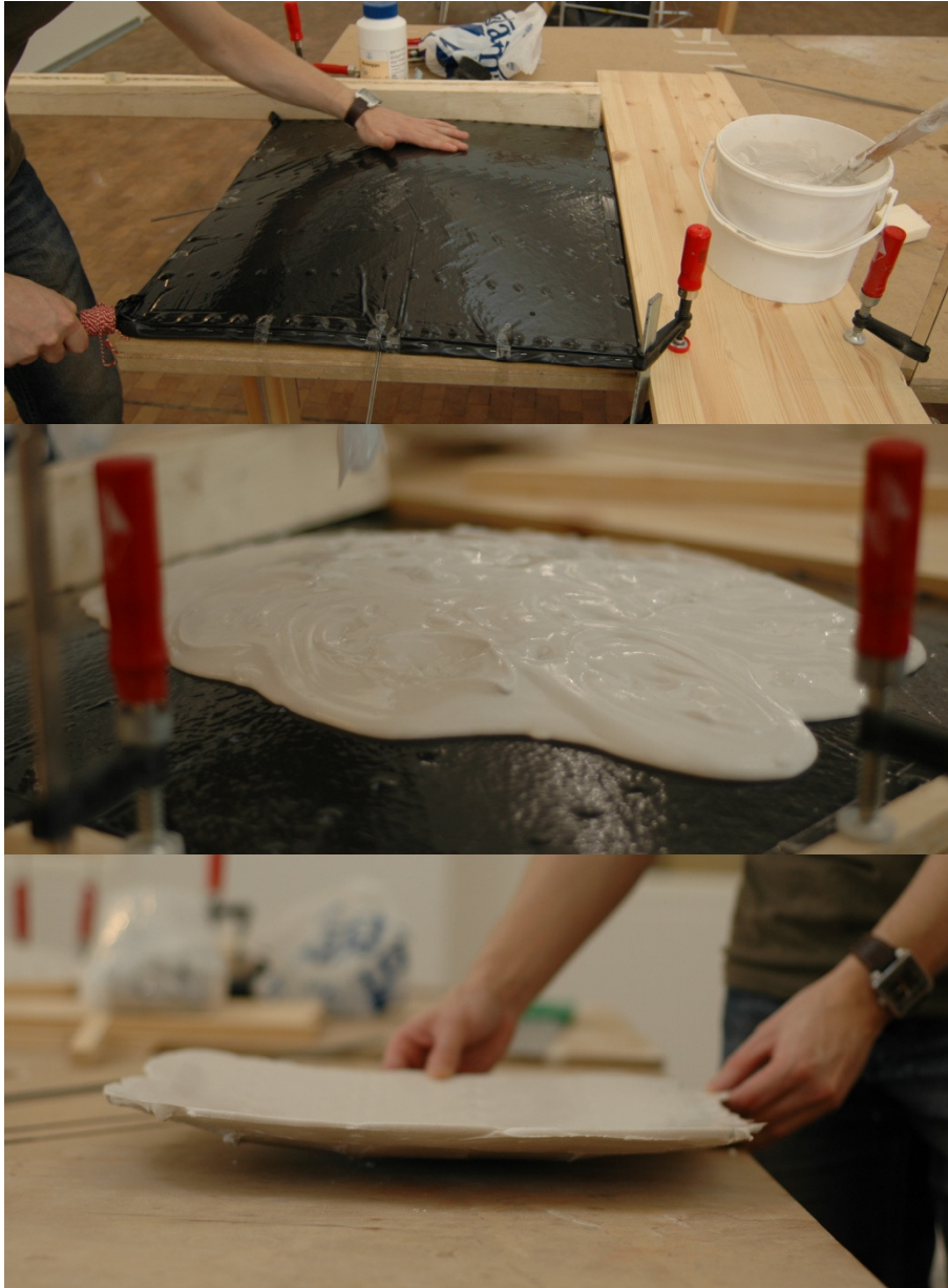
Fig. 8: Pictures from testing the membrane principle. The membrane is fixed to the table around the edges, and supported by a single 6cm high rod in the center. The curvature can be seen to be evenly distributed around the support, and the membrane has a smooth curved cross section over the point support.
