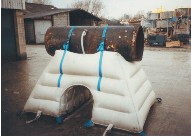
Fig. 16. Fabric-formed pyramidal support for pipeline. Reproduced by permission of FoundOcean, Rebecca Morgan
