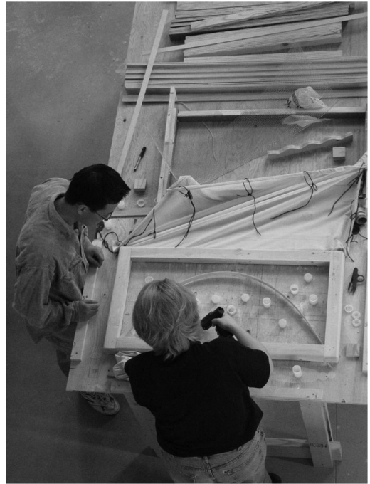
Figure 5. Model wall panel formwork (C.A.S.T. photo).
