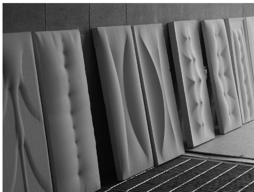
Figure 6. Completed plaster cast wall panels (C.A.S.T. photo).
