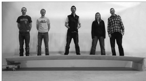
Figure 15. Completed double curvature funicular thin-shell vault (C.A.S.T. photo).
