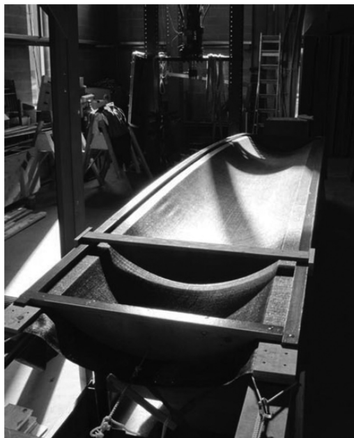
Figure 14. Fabric mold stretched lengthwise in frame to form double curvature funicular thin-shell vault (C.A.S.T. photo).
