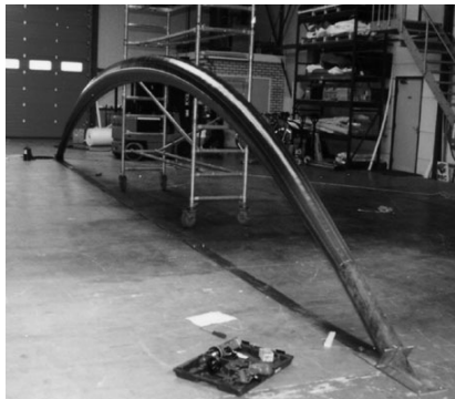
Figure 9: Pneumatic mould supported by the auxiliary structure (Tentech / Buitink Zeilmakerij).
