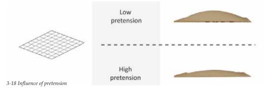
In theory, not only the intensity, but also the form class can be manipulated if it is possible to adjust the pretension locally. This would require a complex mould though, and has not been researched in this thesis.
