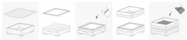
4-4: Process of casting plaster samples
