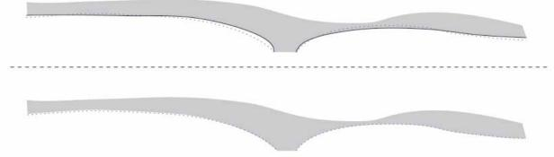
deformed version of that outline. The aesthetic appeal of both versions is the same. This example demonstrates that it is not necessary to construct every point of a free form exactly according to the design; tolerances are high.
