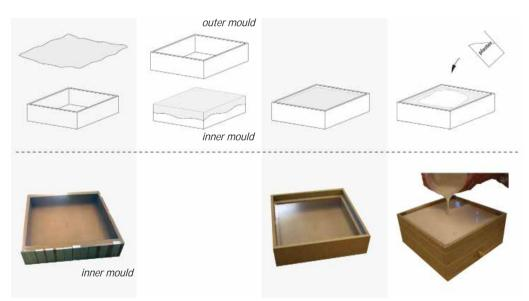
3-6: Process of casting plaster sample
