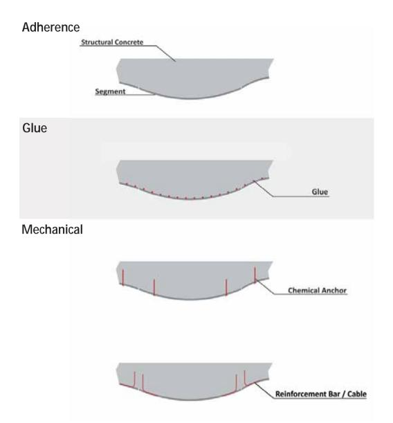
5-4: Schematic display of possible connections between segment and structural concrete
