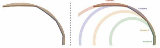
3-19: Curvature of plaster samples can be controlled by adjusting the span of the mould
