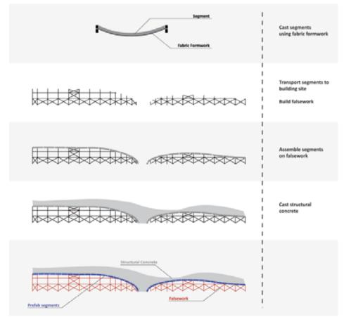
2-18: Building process with prefabricated fabric formwork
