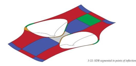
Note: If a free form is segmented 'manually', a number of sections have to be analyzed, its bending points should be marked, after which the bending points have to be connected to obtain the segmented surface. This process is mathematic in its nature. Therefore, the process of segmenting a free form is suitable for computerization by writing an algorithm. Such an algorithm would enable designers to segment a free form with the push of a button.
