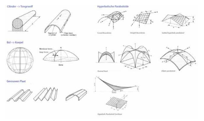
The majority of the shells were constructed by pouring concrete onto a wooden formwork. The construction of this formwork required a large workforce of experienced craftsmen. Complex double-curved forms could be subdivided into linear elements, which made it possible to construct a formwork out of straight boards.
