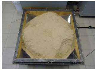
4-22: Top mould is loaded with sand
