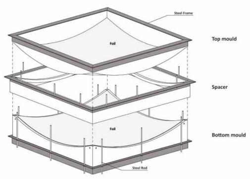
4-11: Exploded view of the mould
