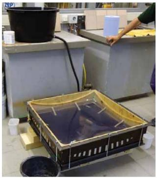
4-19: Filling the bottom mould with water
