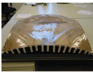
4-34: Plastic deformations in foil (before restretching)
