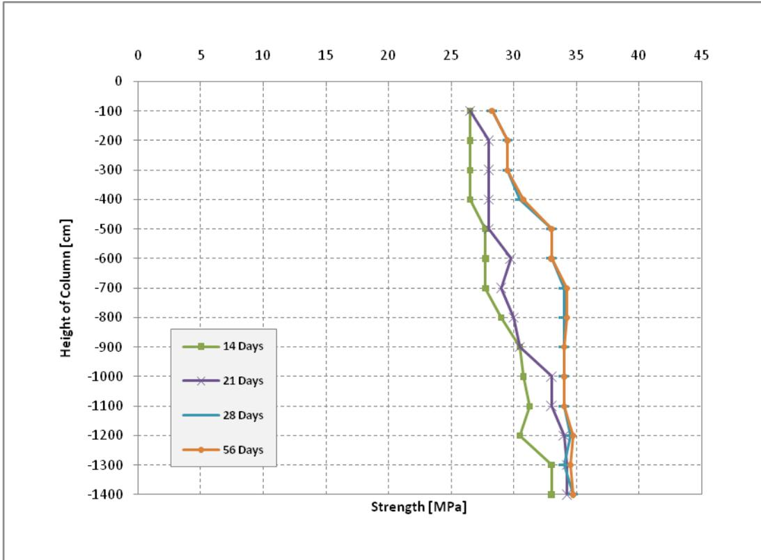
Figure C4: Column C4 – Cardboard Tube, Flyash Concrete
