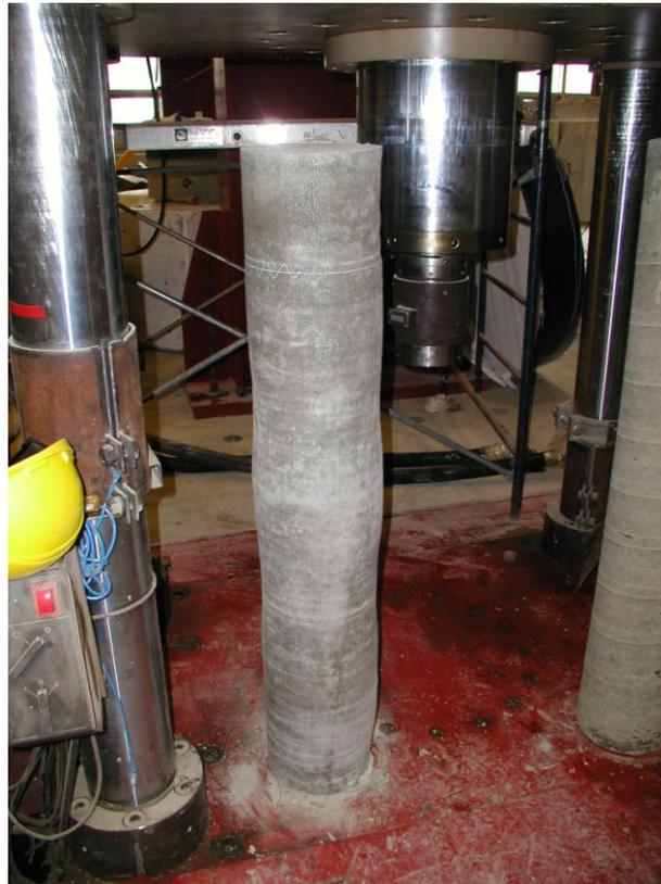
Figure 67: Bulged concrete column
