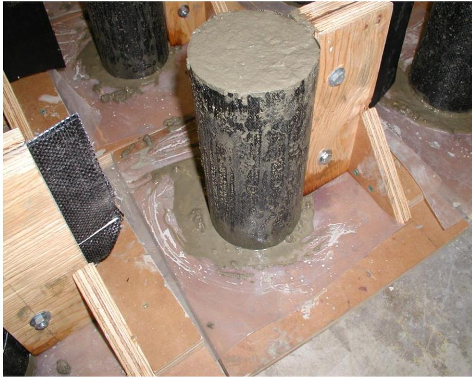
**Figure 34: Fabric-formed concrete cylinders**
