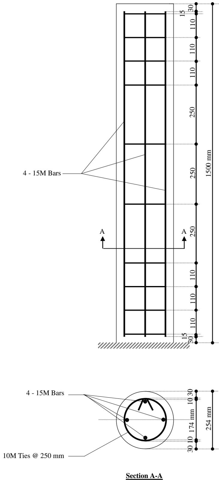
Figure 42: Column reinforcement details
