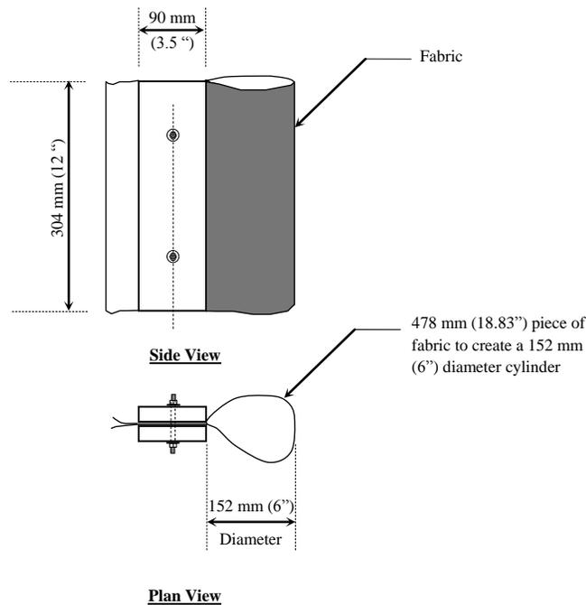
Figure 19: Details of fabric mold for concrete cylinders
