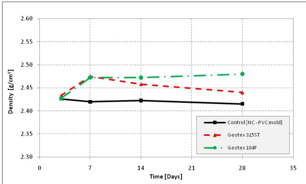
Figure 38: Average density of normal concrete cylinders
