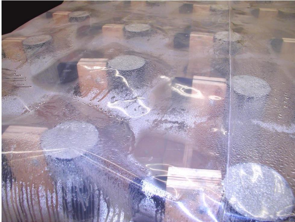
Figure 36: Cylinders curing
