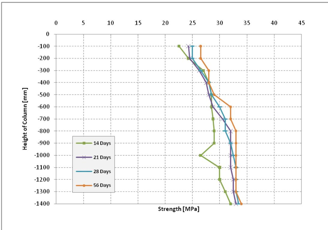
Figure C5: Column C5 – Fabric Formwork, Normal Concrete
