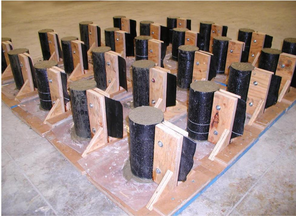
**Figure 35: Fabric-formed cylinders after casting**
