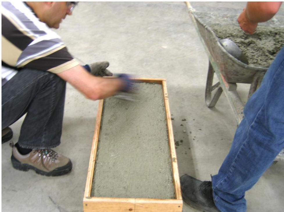
Figure 9: Filling the box with fresh concrete
