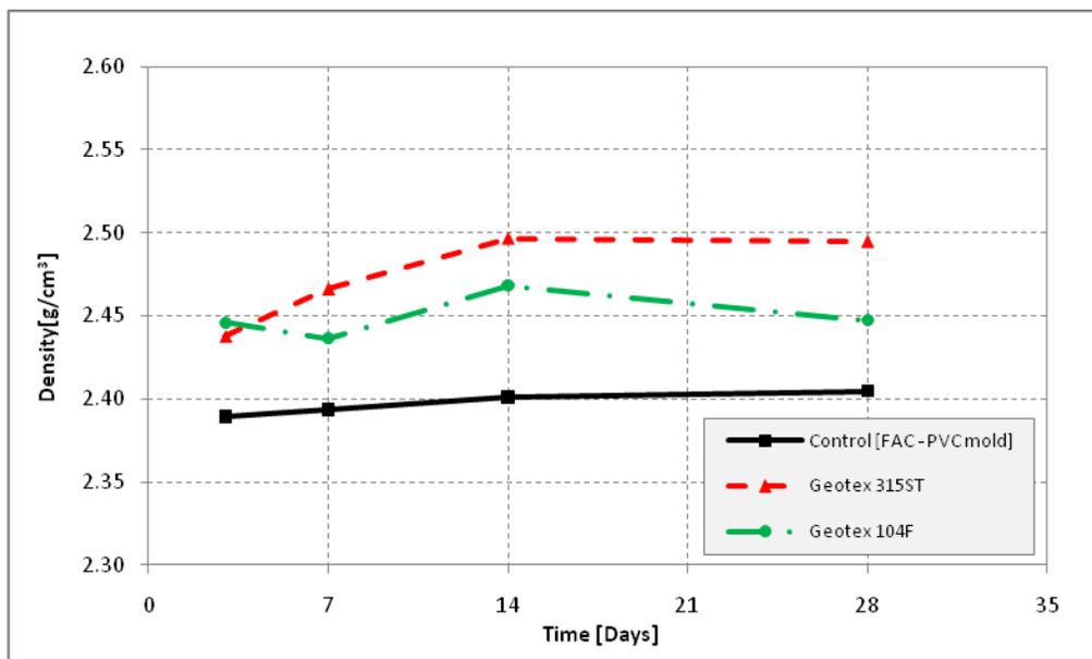
Figure 39: Average density of flyash concrete cylinders
