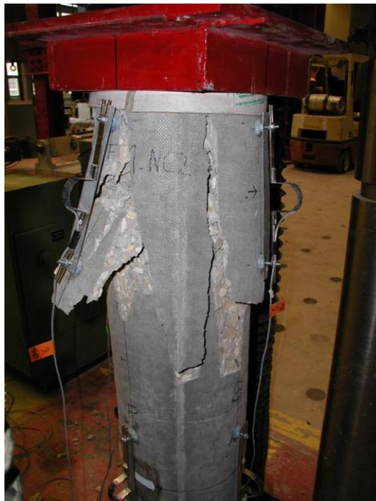
Figure 64: Column FF-NC-2 after failure
