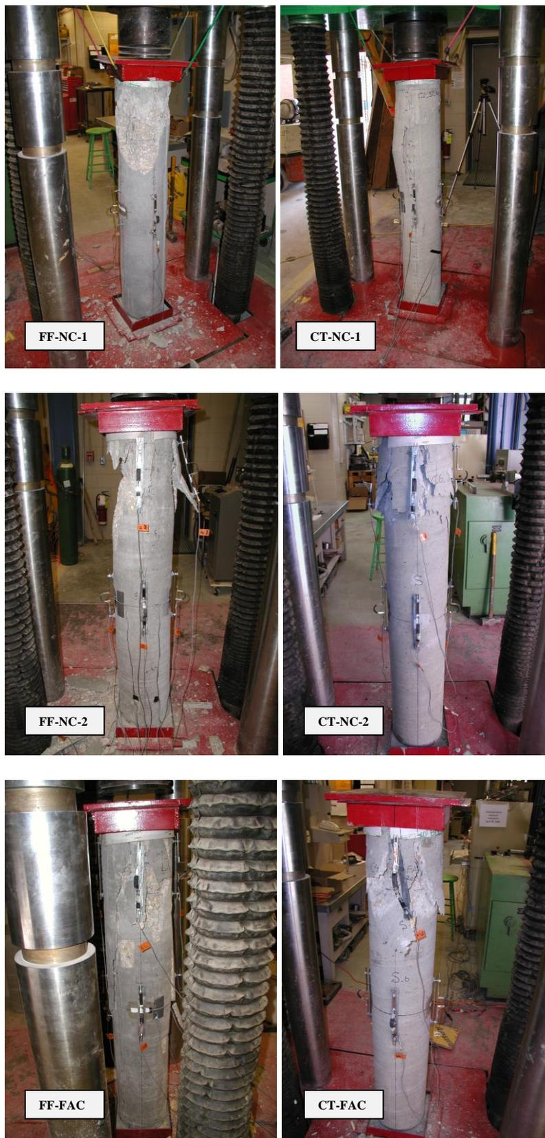
Figure 65: All columns after failure
