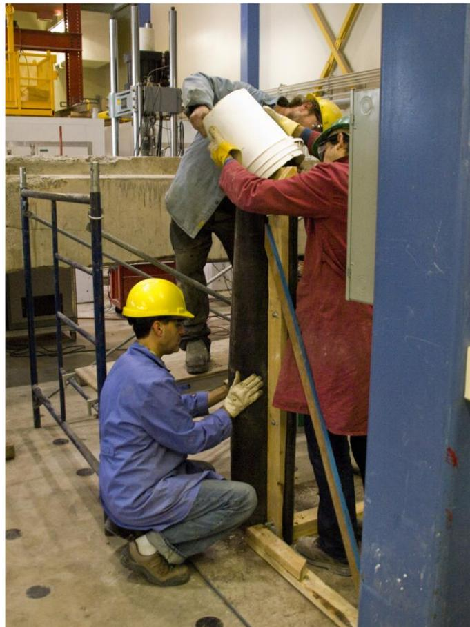
Figure 47: casting of column in fabric formwork
