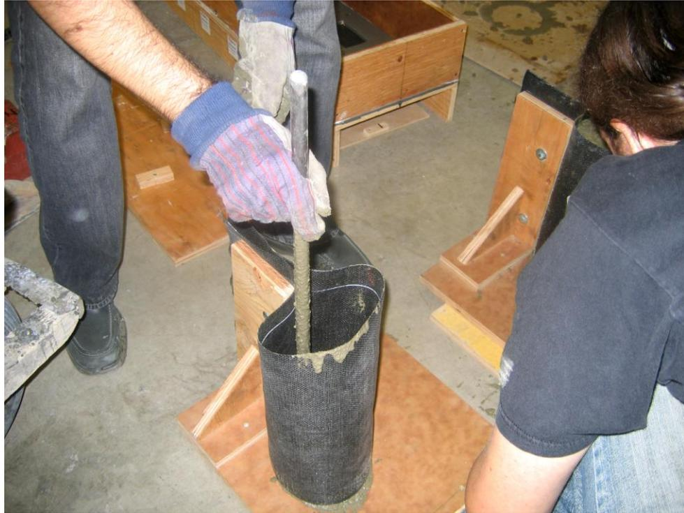
Figure 21: Compacting fresh concrete using the standard rod
