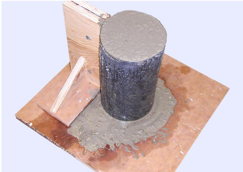
Figure 22: Fabric mold filled with fresh concrete
