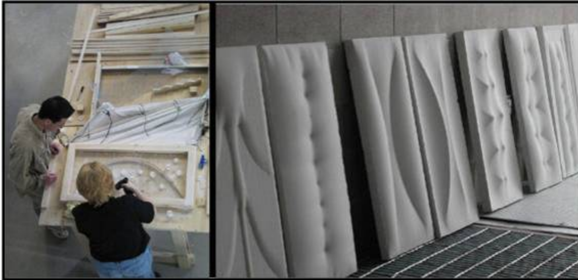
Fig. 1. Model formwork and completed plaster cast.
