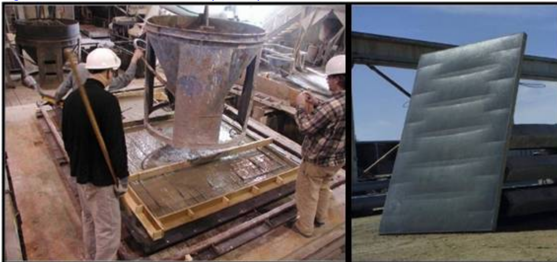
Fig. 2. Full-scale formwork and completed concrete panel.
