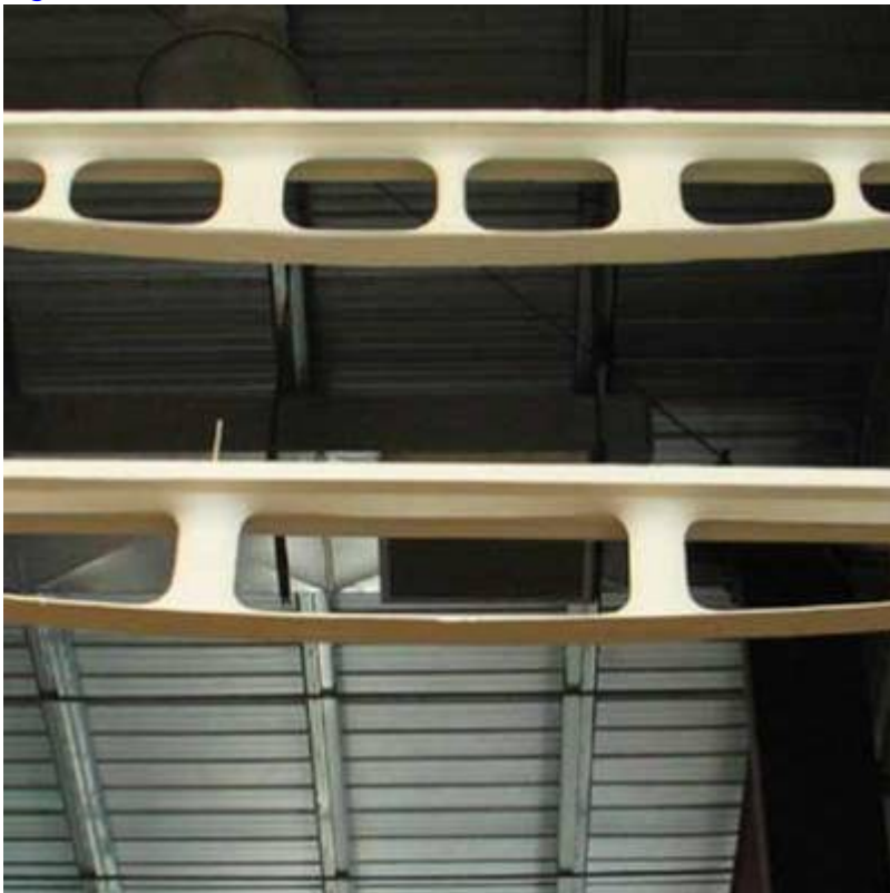
Fig. 4. Completed truss plaster casts.
