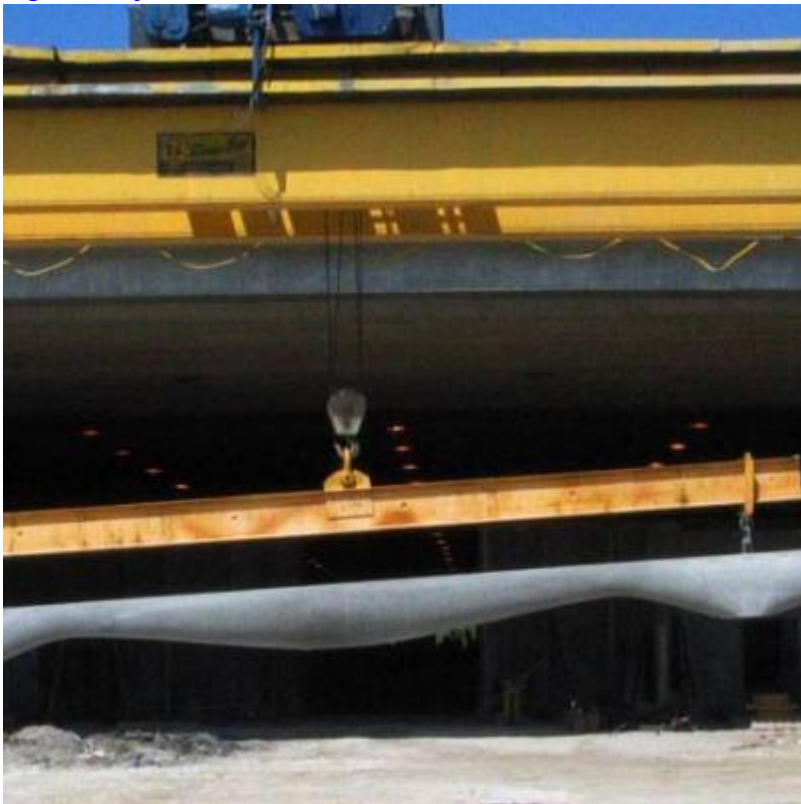
Fig. 12. Completed full scale variable section concrete beam.
