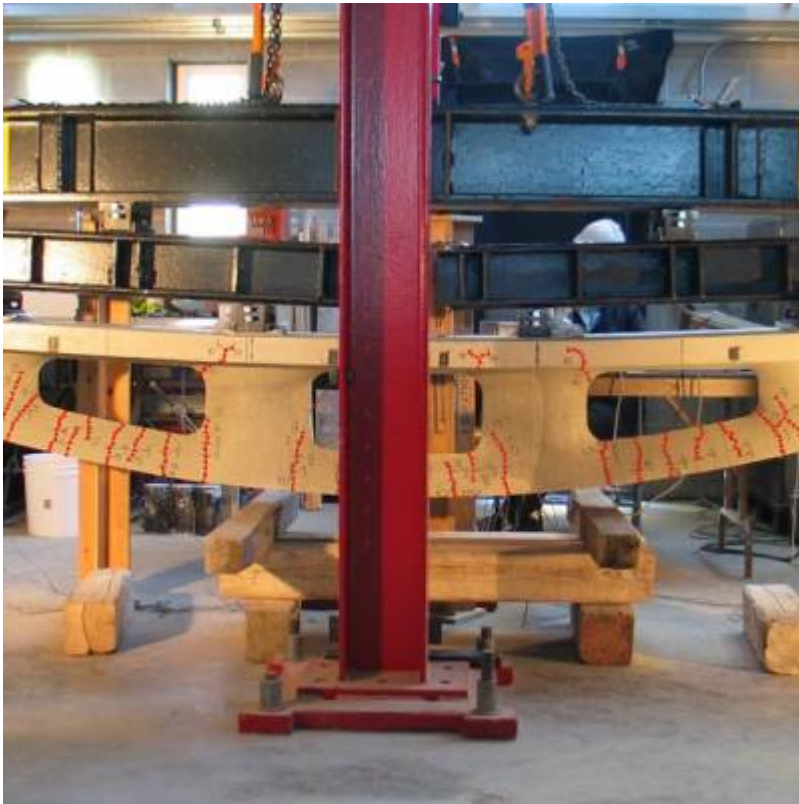
Fig. 15. Testing of variable section concrete truss.
