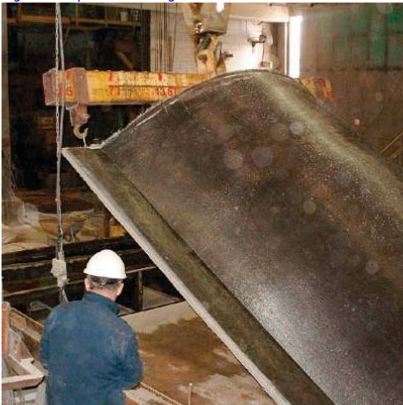
Fig. 25. Step 4 - Thin-shell funicular GFRP vault produced from mold.
