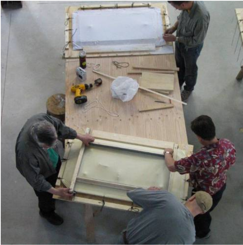
Fig. 2. Model wall panel formwork.
