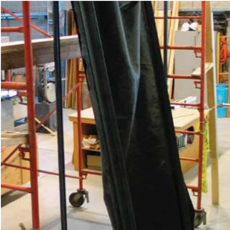
Fig. 45. Hanging sheet of polyolefin geotextile used as mold to produce...
