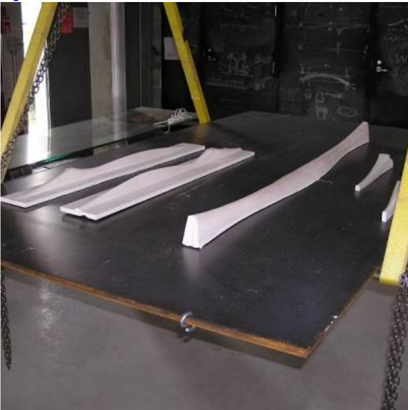
Fig. 2. Completed beam plaster casts.
