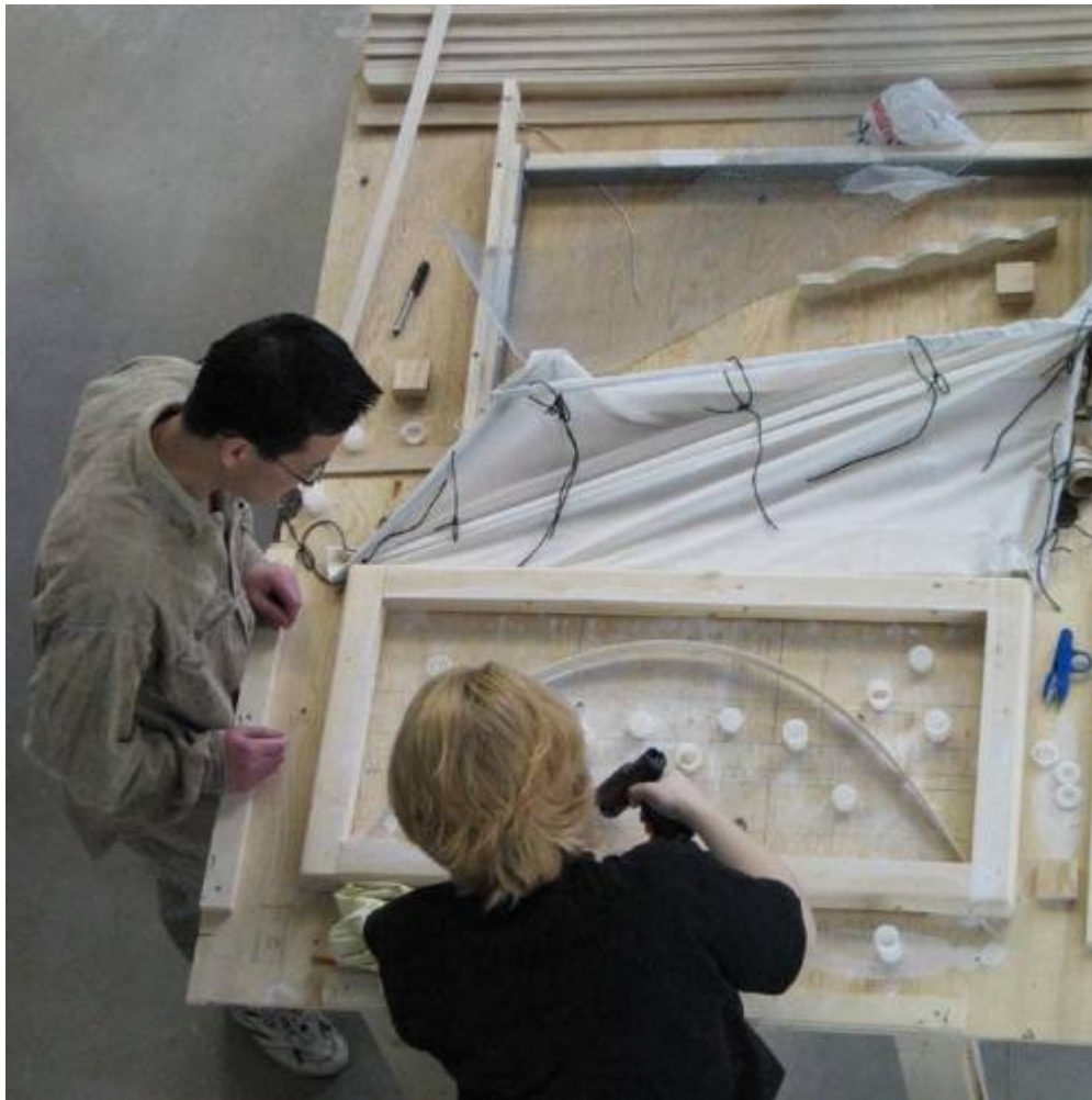
Fig. 1. Model wall panel formwork.
