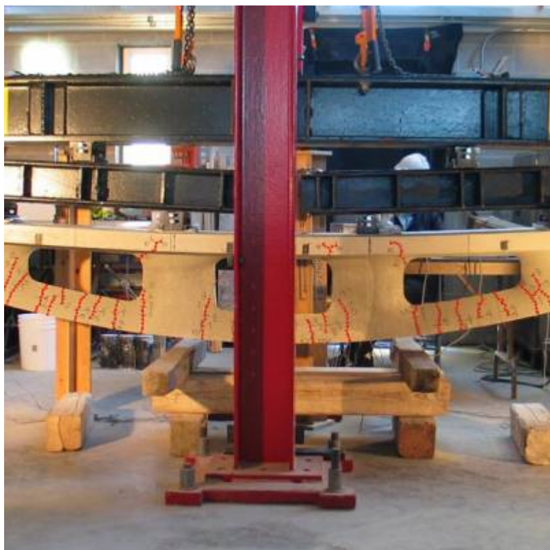
Fig. 15. Testing of variable section concrete truss.
