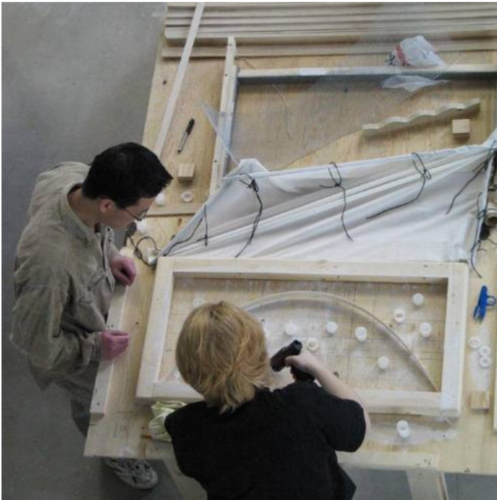
Fig. 1. Model wall panel formwork.
