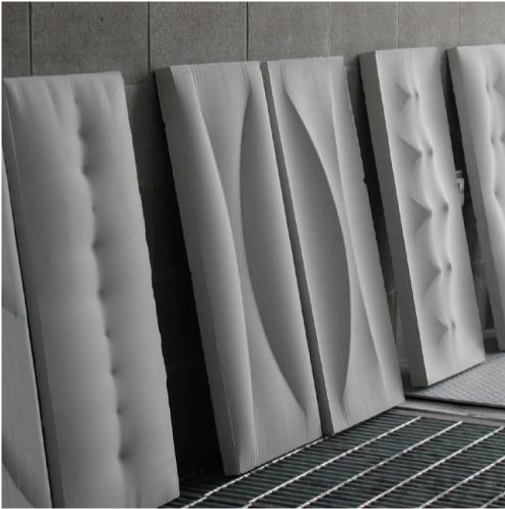
Fig. 3. Completed wall panel plaster casts.
