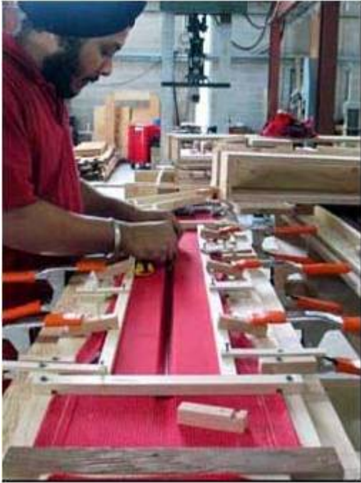
Fig. 1. Model beam formwork.
