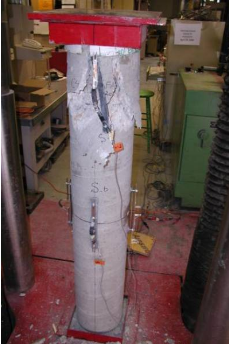
Figure 65: Column CT-FAC after failure.
