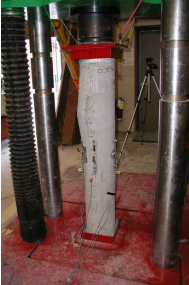
Figure 65: Column CT-NC-1 after failure.
