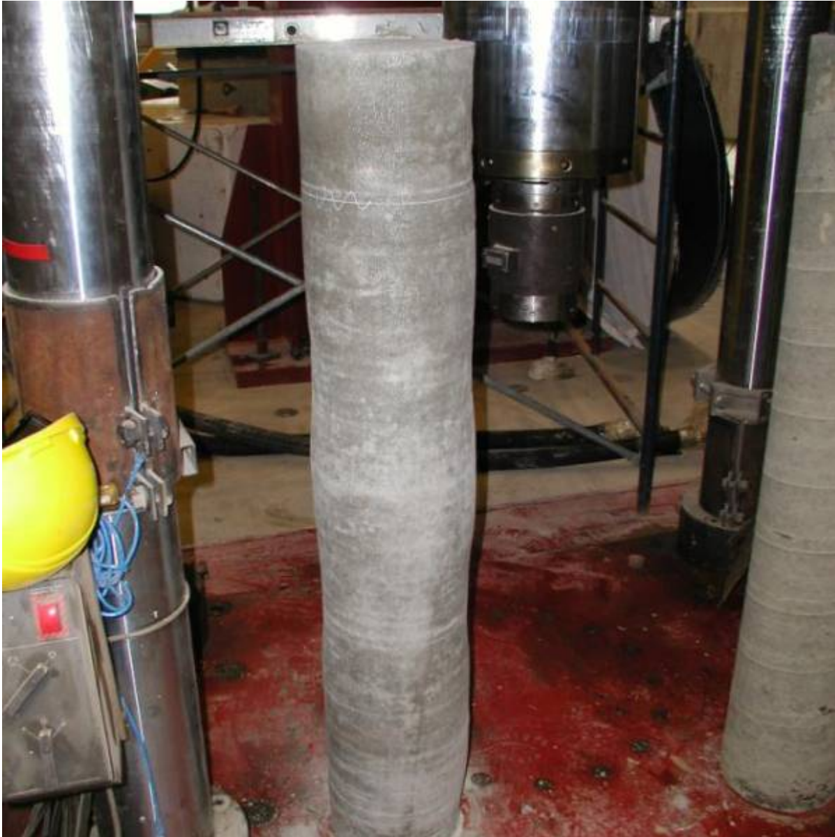
Figure 67: Bulged concrete column.
