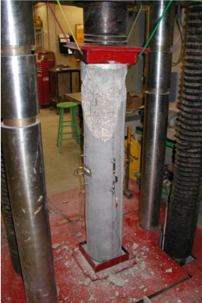
Figure 65: Column FF-NC-1 after failure.
