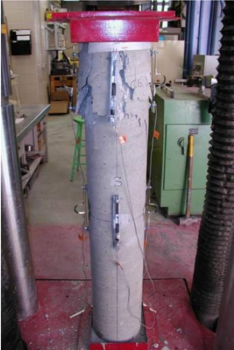
Figure 65: Column CT-NC-2 after failure.
