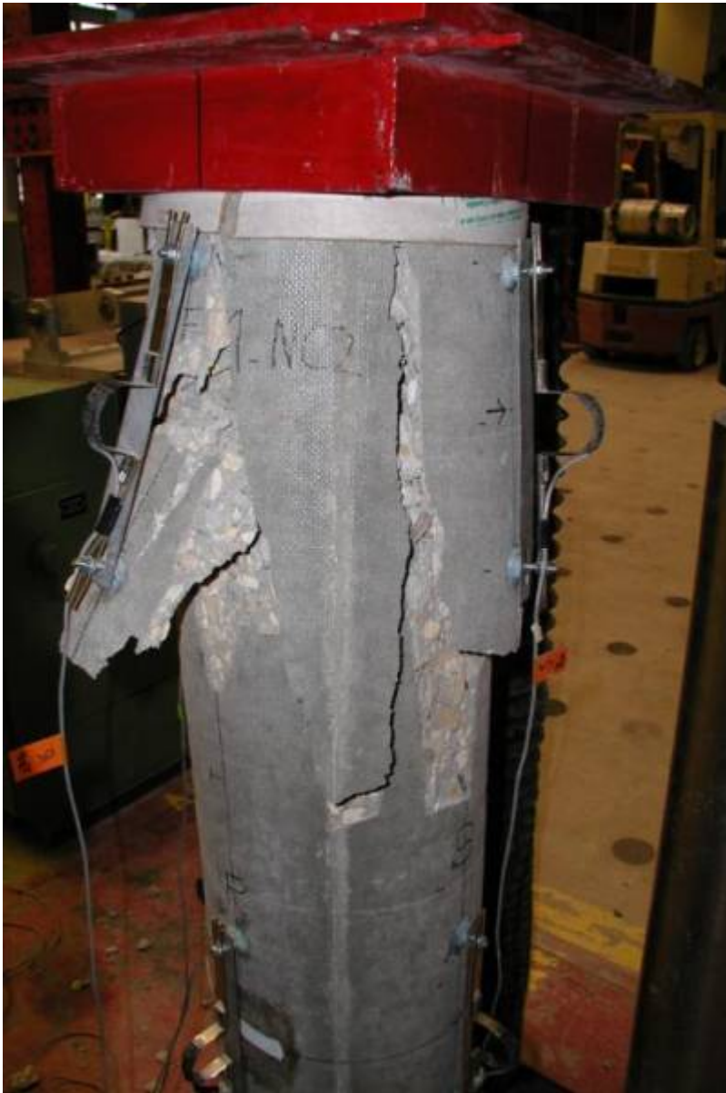
Figure 64: Column FF-NC-2 after failure.
