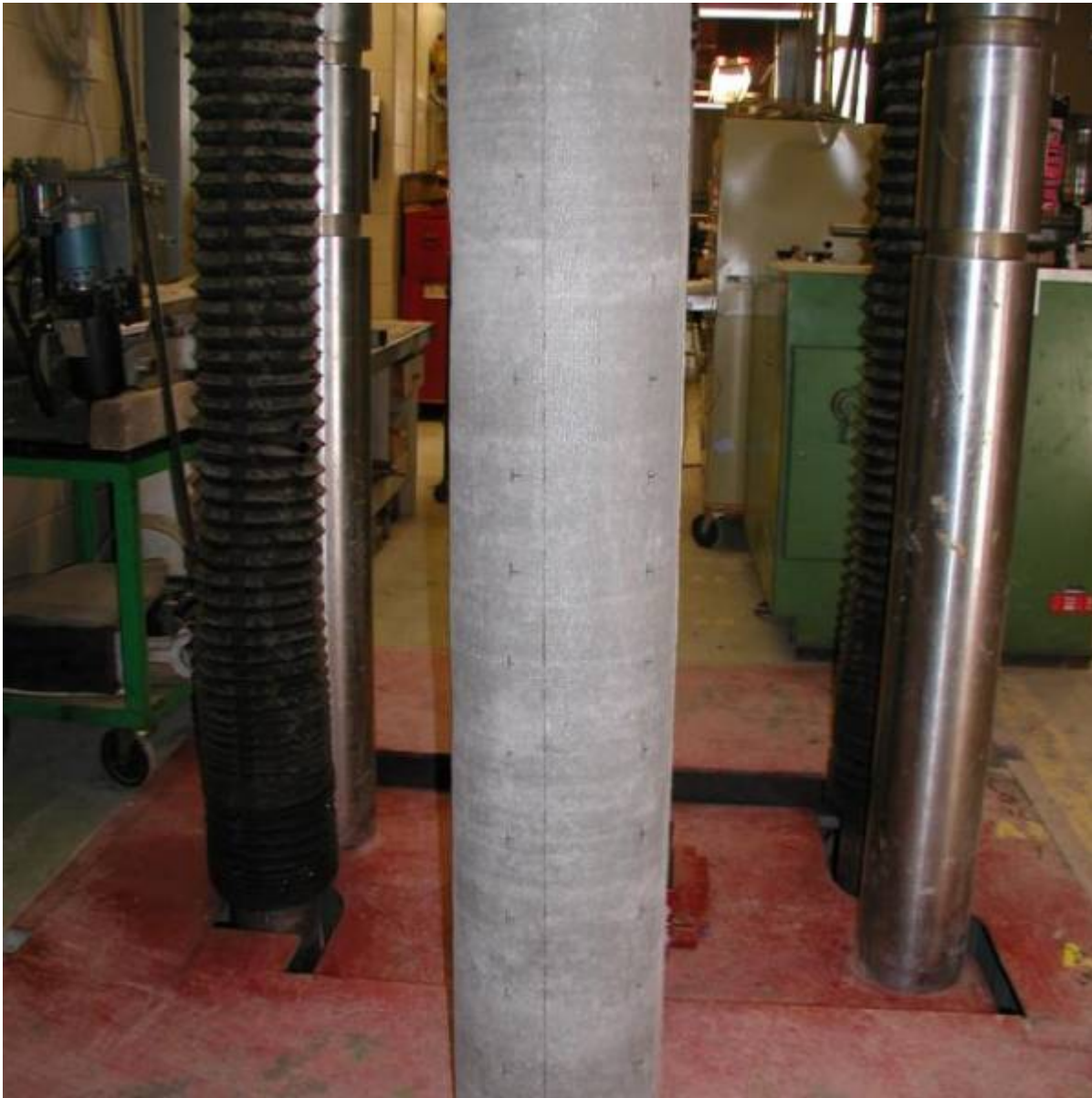
Figure 68: Modified fabric formwork resulting in a straight column.
