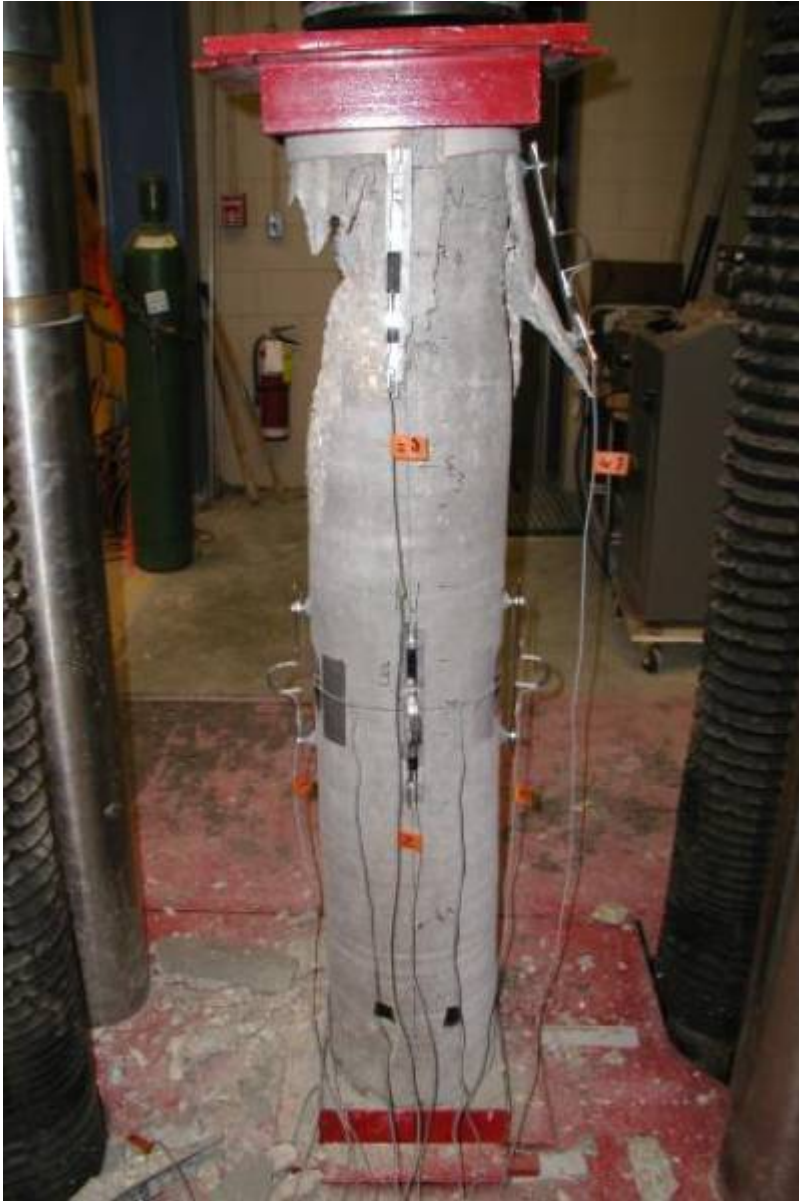
Figure 65: Column FT-NC-2 after failure.
