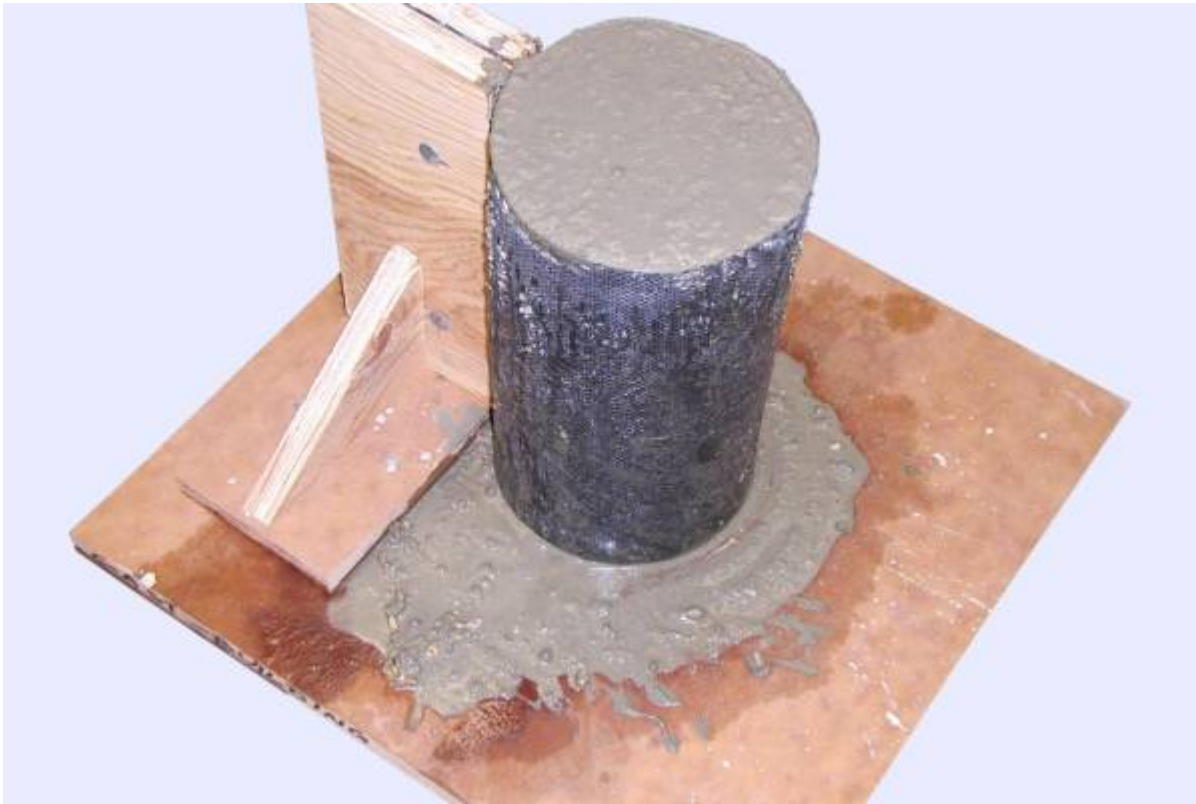
Figure 22: Fabric mold filled with fresh concrete.
