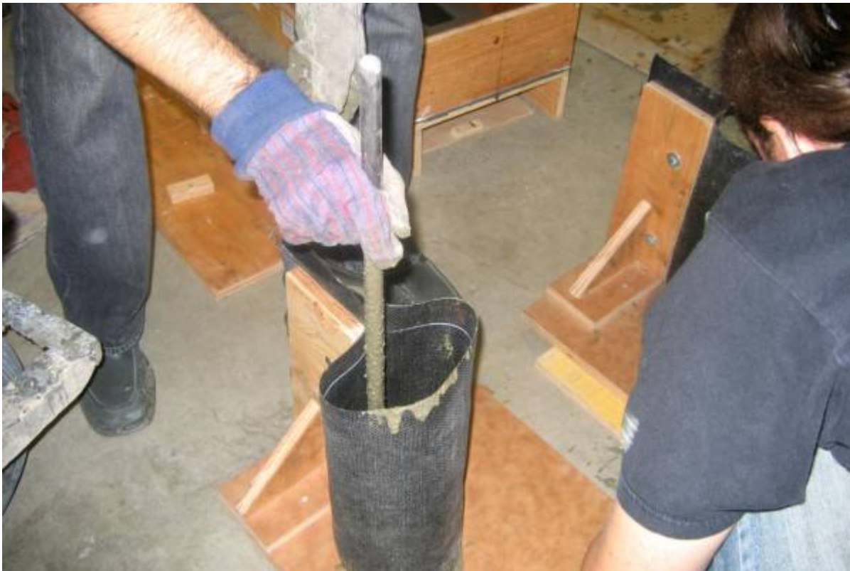
Figure 21: Compacting fresh concrete using the standard rod.
