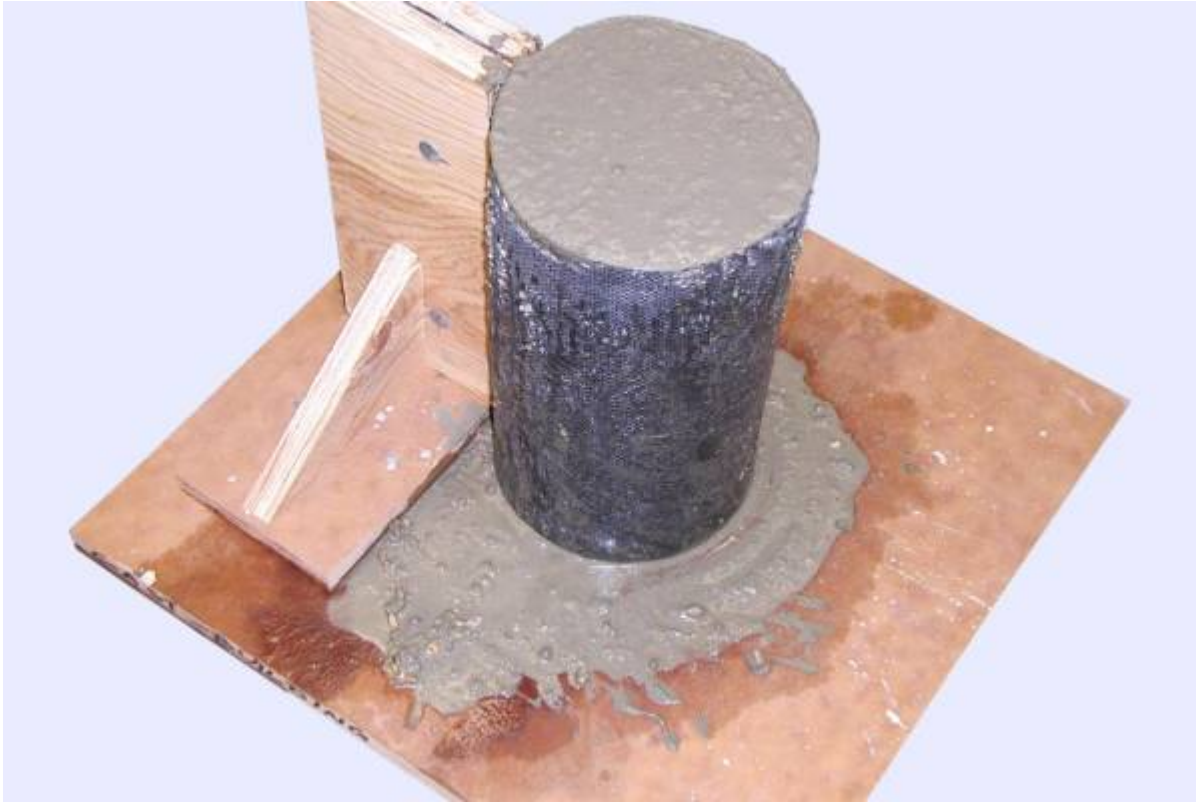
Figure 22: Fabric mold filled with fresh concrete.
