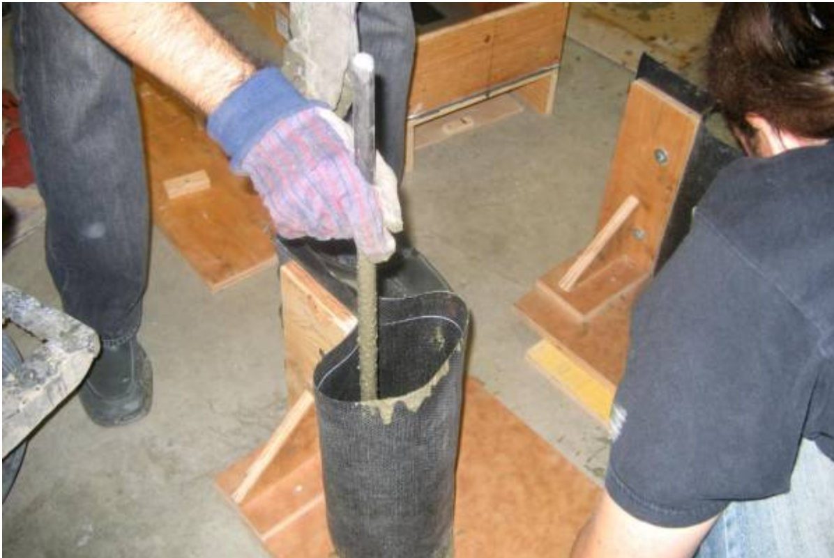
Figure 21: Compacting fresh concrete using the standard rod.
