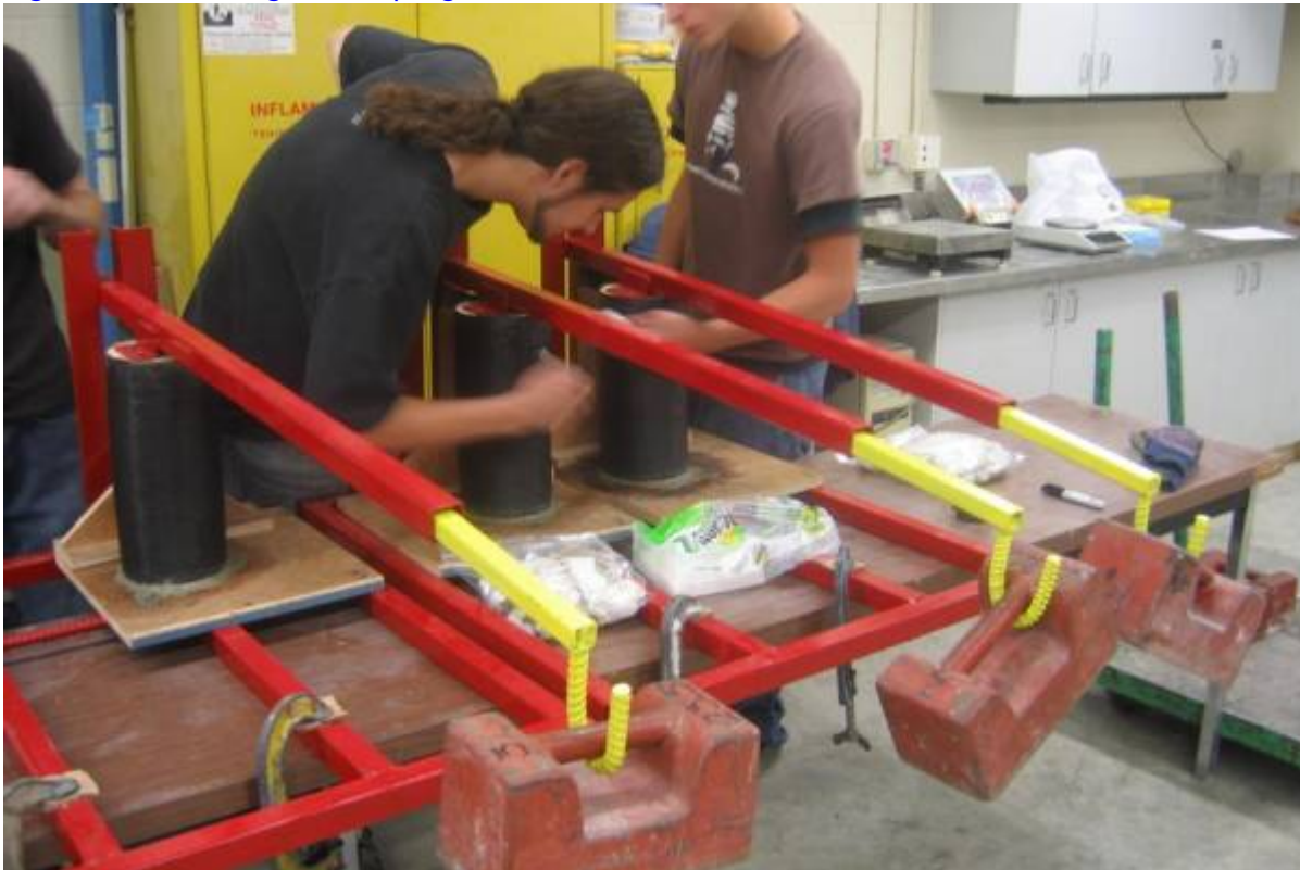
Figure 29: Collection of bleeding water during the bleeding test.
