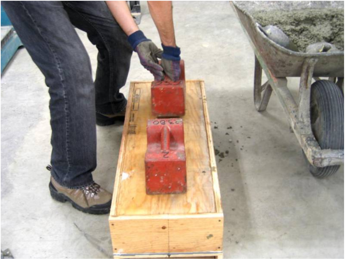
Figure 10: Extra pressure on fresh concrete to accelerate the bleeding process.
