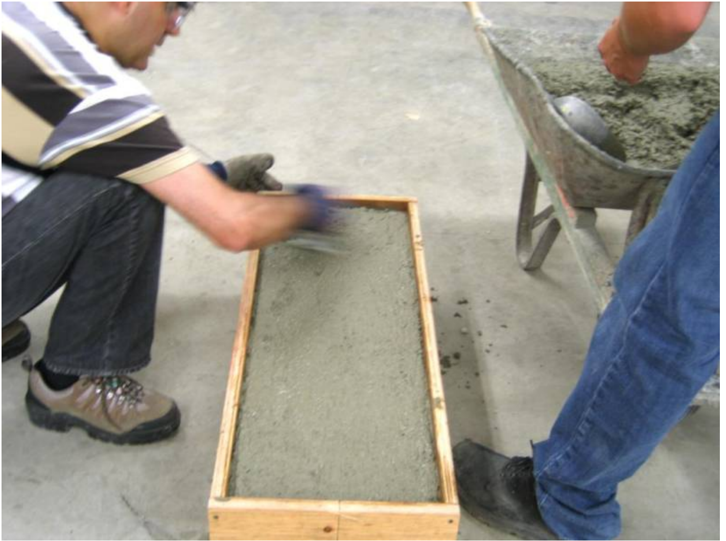
Figure 9: Filling the box with fresh concrete.
